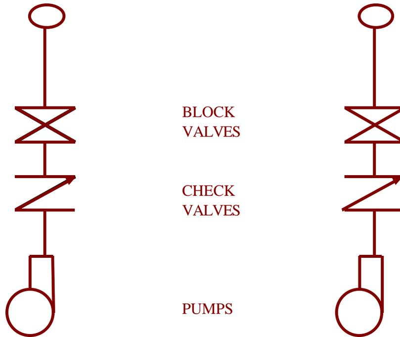
**SYSTEM:** A check valve is used for pump protection to insure backflow doesn't damage the pumps.
