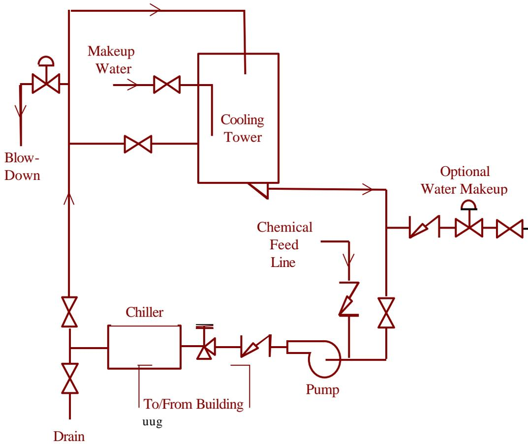
**SYSTEM:** A typical single cell cooling tower installation provides chilled water to a building, plant or hospital. The basic components of the system are a circulating pump, a chiller and the cooling tower along with the associated valving, piping and control equipment.
