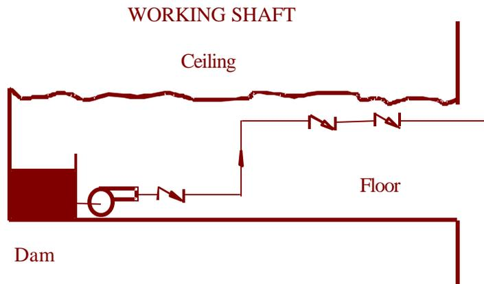
**Long Horizontal Pipe Runs:** If the check valves do not provide tight sealing, the entrained air that separates from the water during shut-down can leak past the check valve. This can cause significant air pockets to form. Since there is little or no back pressure on the swing checks, they will allow the air to bleed past the valve causing large air pockets to develop. Water hammer and its associated damage is then a very common problem during start-up.
