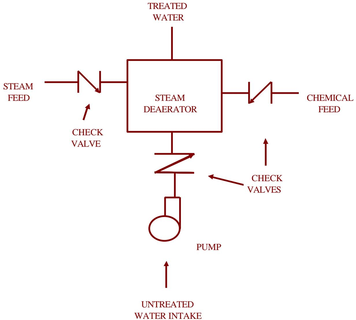
**SYSTEM:** Typically in a steam plant water has oxygen removed before entering the boiler to prevent boiler corrosion. This is accomplished by adding chemicals and steam to the water.
