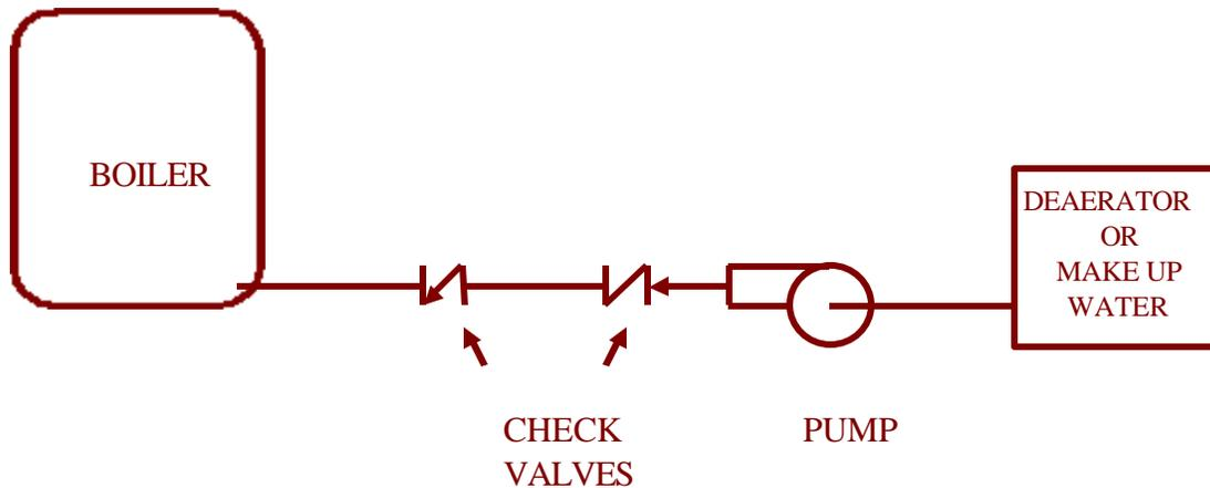
**SYSTEM:** All steam boilers have a need for intermittent water flow to replace the water generated into steam to feed the system.
