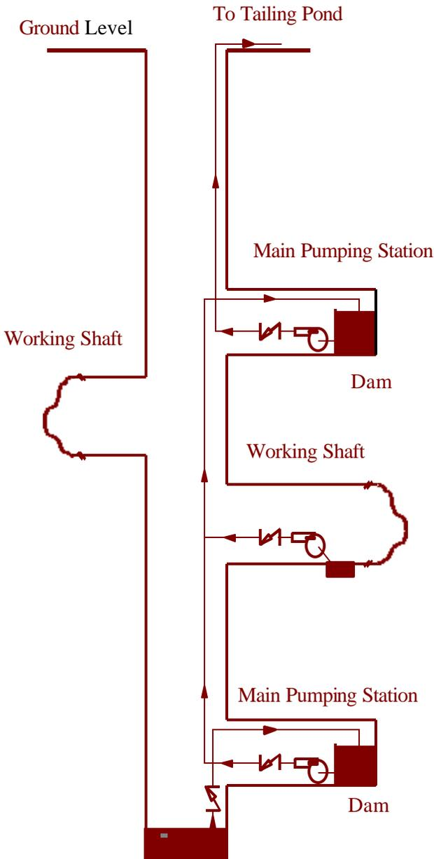
**SYSTEM:** During underground mining, there is usually a large amount of water that collects in the mine shafts. This water comes from underground springs that flow through the walls and from water that is pumped into the mine for operational use. All of this water needs to be removed.
