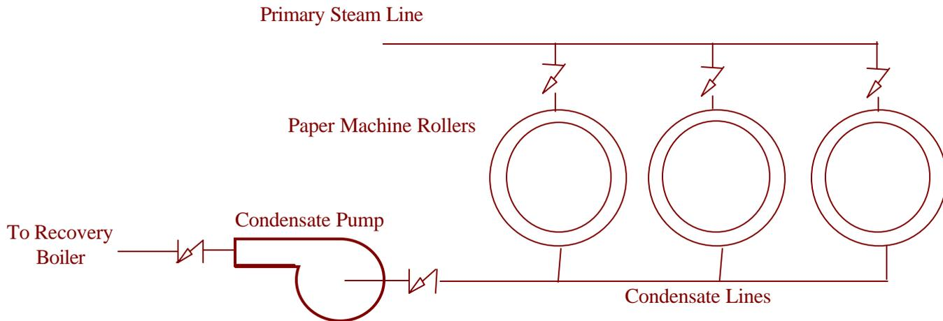
**SYSTEM:** Pulp is passed through the fourdrinier machine to produce paper. After the fourdrinier, the paper moves to the paper machine roller. The roller is a series of steam-heated rollers that remove most of the remaining water from the paper. The paper moves over and under these rollers. These rollers are used to insure that the paper finishes with the correct moisture content.
