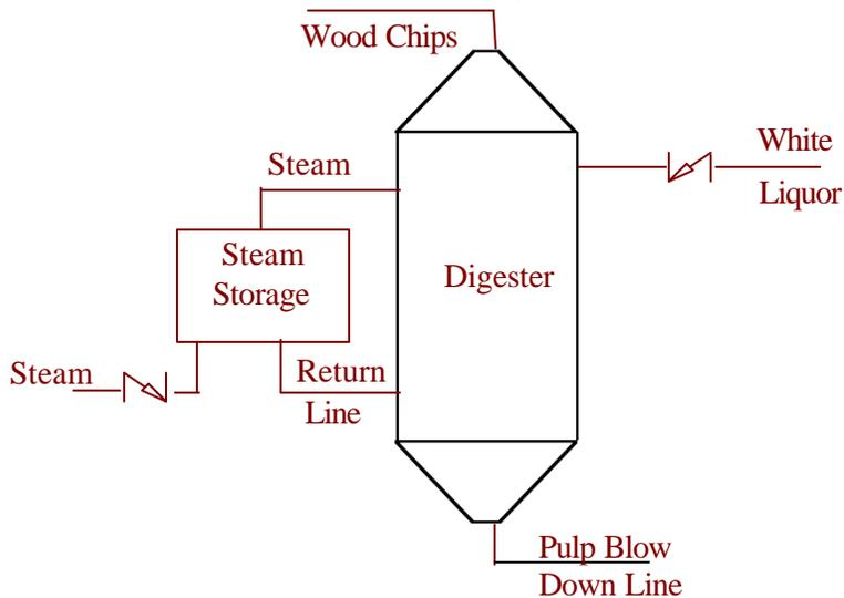
**SYSTEM:** A digester is a large piece of equipment that cooks wood chips and produces the raw pulp. Steam and White Liquor are added to the wood chips to produce the raw pulp. After they are reduced to pulp, the pulp is “blown” out of the digester. The digester is similar in operation to a large pressure cooker. Digesters range in size from 10-20 feet in diameter and 40-70 feet high. They usually operate at pressures up to 150 psi.
