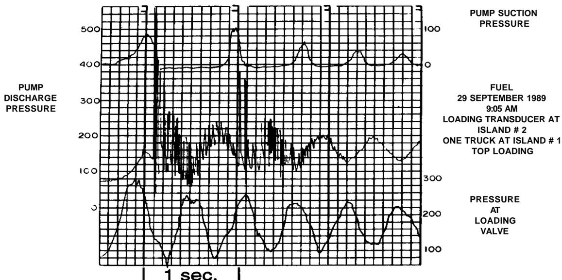
Experience indicated to the consultant that this water hammer occurred due to the use of a swing check valve on the discharge of the pump. A swing check closes fairly slowly and allows back flow to occur. When the valve finally closes, the back flow is abruptly stopped, causing extremely rapid pressure build-up (water hammer).
