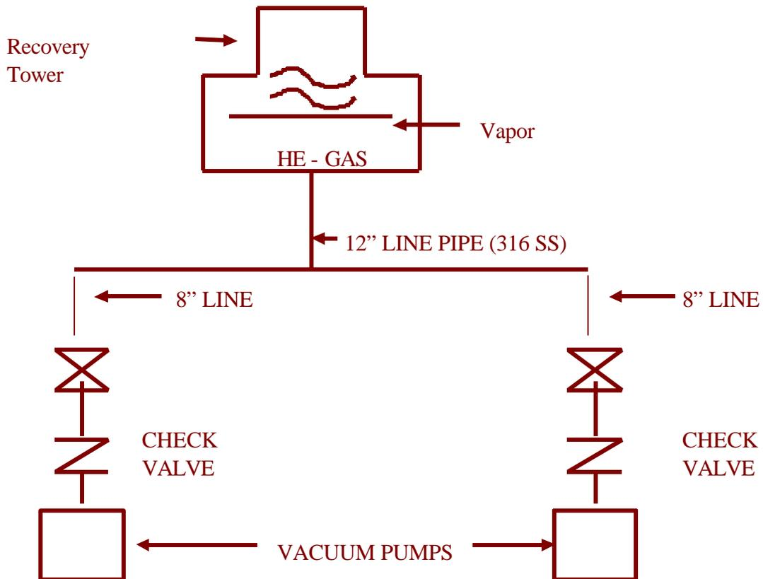
**SYSTEM:** Helium gas vapor recovery system by process of a vacuum suction. The object of the check valve is to prevent flow from being sucked by vacuum towards the recovery tower.
